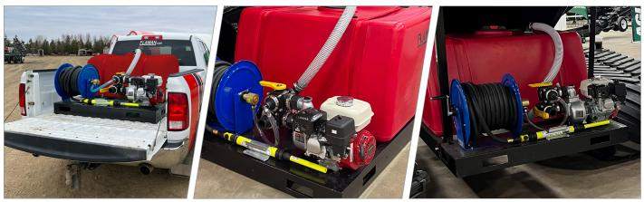
Built-in fork pockets allow you to easily move the 48" wide skid to your half-ton truck or grain cart.
